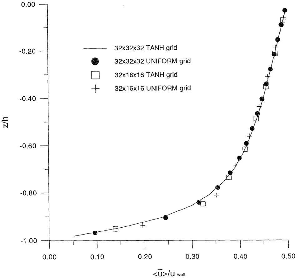
Fig. 2a The effect of grid resolution on the mean velocity profile
