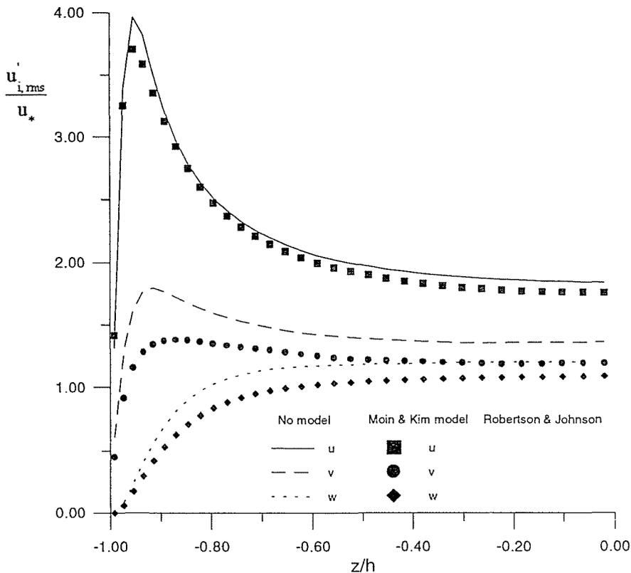
Fig. 4b Comparison of simulations and experiment (mean profile and intensities)
