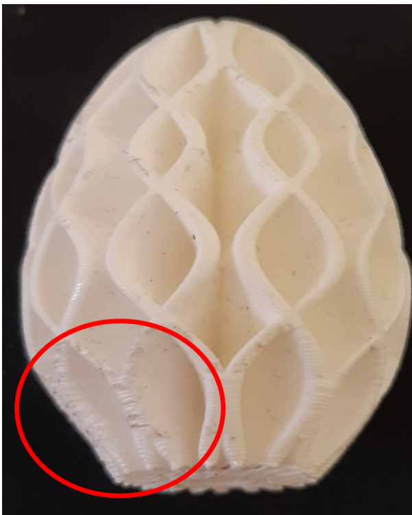
Fig. 1 The surface error caused by insufficient cooling on the overhangs
