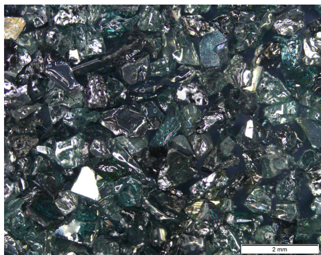
Fig. 2 Macroscopic image of the applied reinforcement particles: 0.6 mm nominal size of SiC
