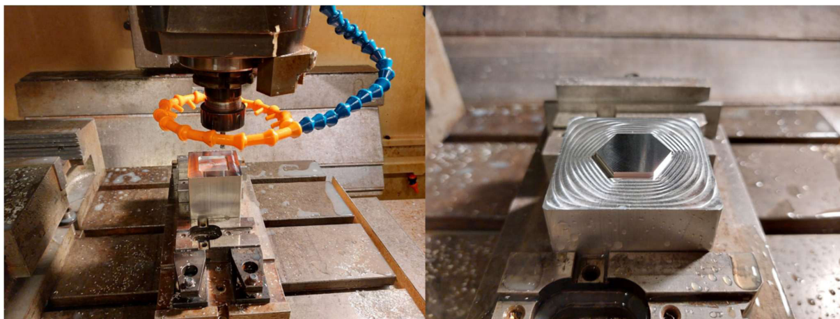
Fig. 3 The experimental setup for cutting tests and a machined hexagonal island shaped by a Lamé curve
