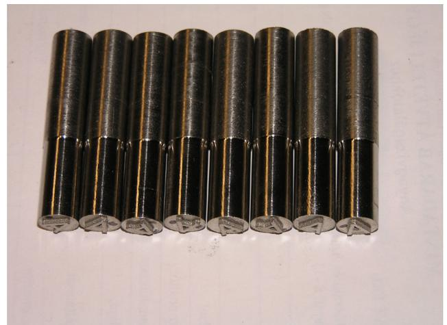
**Fig. 3** Samples before and after postprocessing: The upper part of the picture shows raw surface, and bottom part the burnished surface
