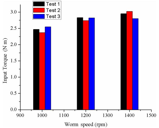
**Fig. 6** Repeatability of churning loss measurement for worm gear pair for Set 2 as per Table 4
