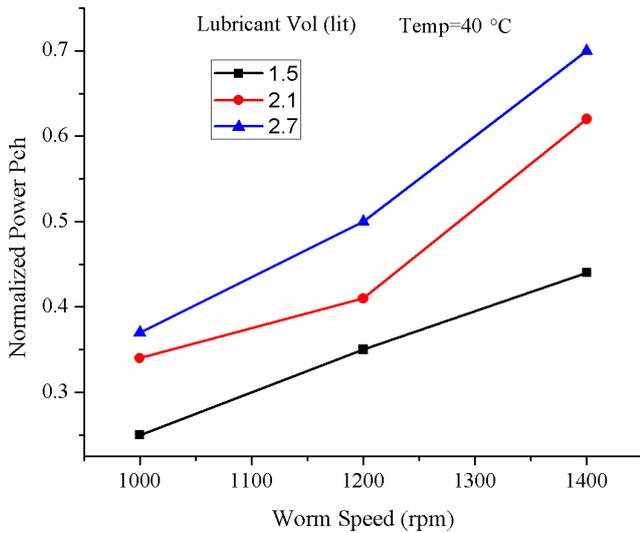
Fig. 7  $P_{ch}$  vs Worm speed @ 40 °C
