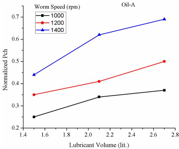
Fig. 11 Influence of worm speed for worm at bottom, 40 °C with Oil-A
