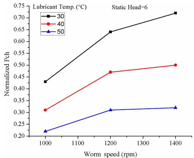
Fig. 10 Influence of temperature for worm at the bottom and Oil-B for static head H = 6
