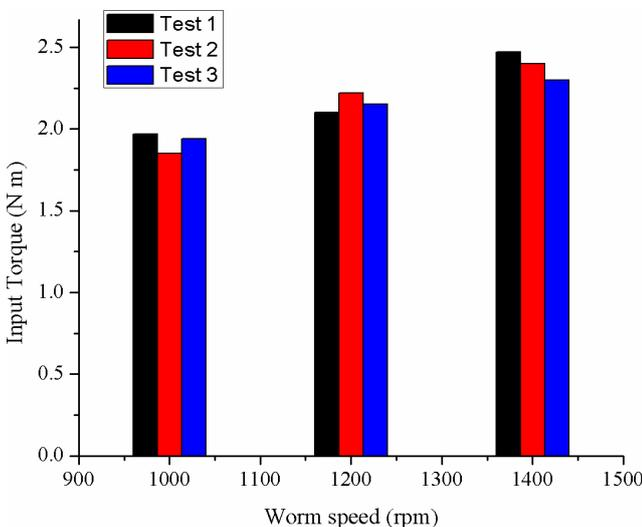
**Fig. 5** Repeatability of churning loss measurement for worm gear pair for Set 1 as per Table 4
