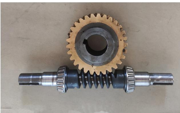
Fig. 3 Single start worm and worm wheel
