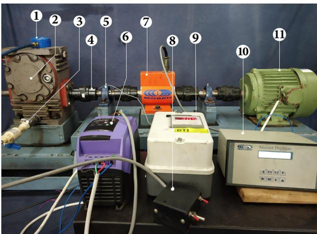
**Fig. 1** Test rig to investigate churning power loss of worm gear;
