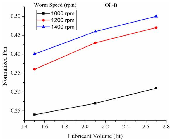
Fig. 12 Influence of worm speed for worm at bottom, 40 °C with Oil-B
