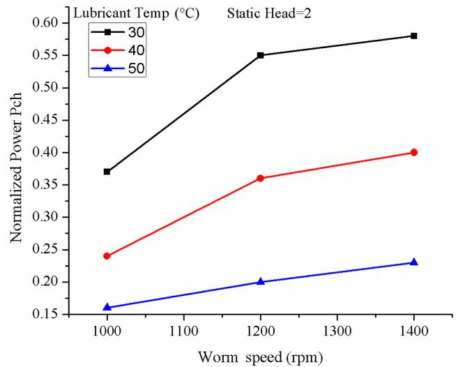
Fig. 9 Influence of temperature for worm at the bottom and Oil-B for H = 2
