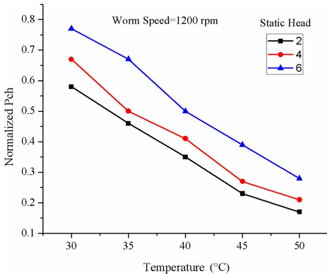
Fig. 8  $P_{ch}$  vs temperature of lubricant @ 1200 rpm
