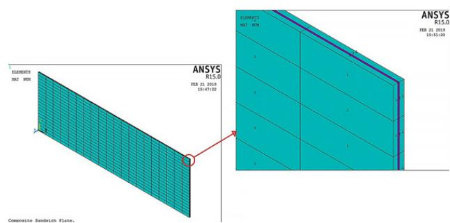
**Fig. 3** Finite element modeling of the composite sandwich plate using the two different element types of ANSYS: adapted from [18]
