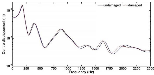
**Fig. 11** Frequency response of simply supported viscoelastic composite sandwich plate in point  $P(L/2, l/2)$  for the undamaged and damaged cases with  $\theta = 0^\circ$
