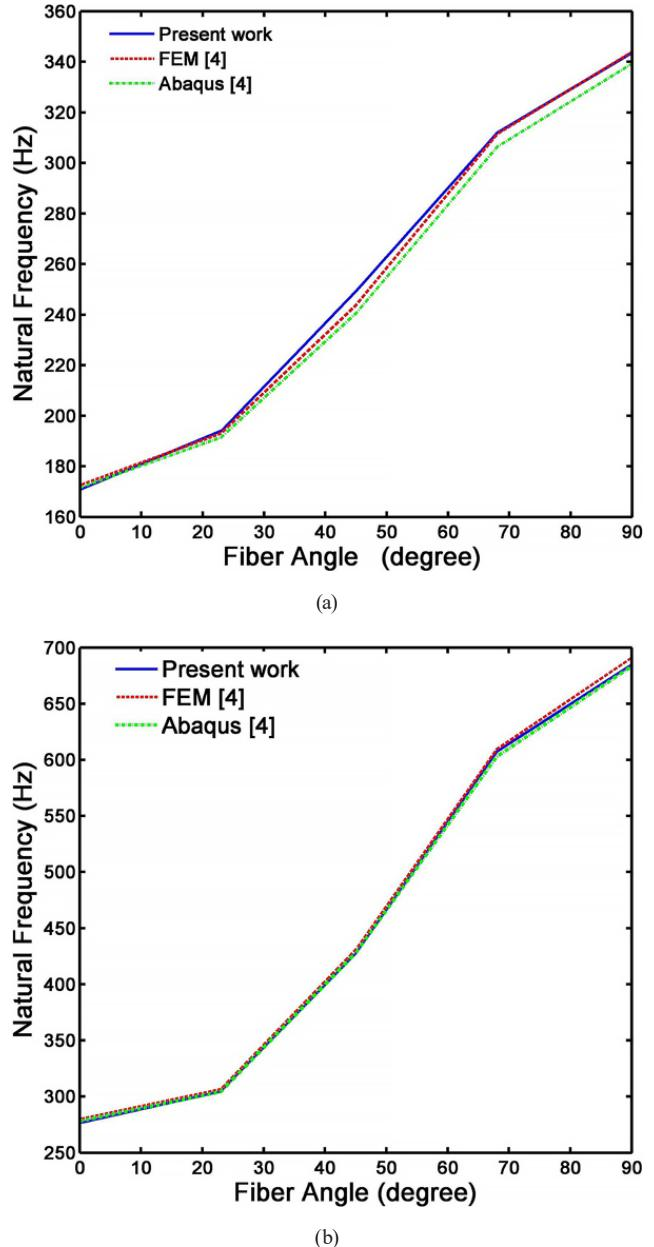
**Fig. 7** Influences of face sheets fiber angle ( $^\circ$ ) of the undamaged viscoelastic composite sandwich plate on natural frequencies of the first mode of vibration: (a) simply supported boundary condition, (b) clamped boundary condition
