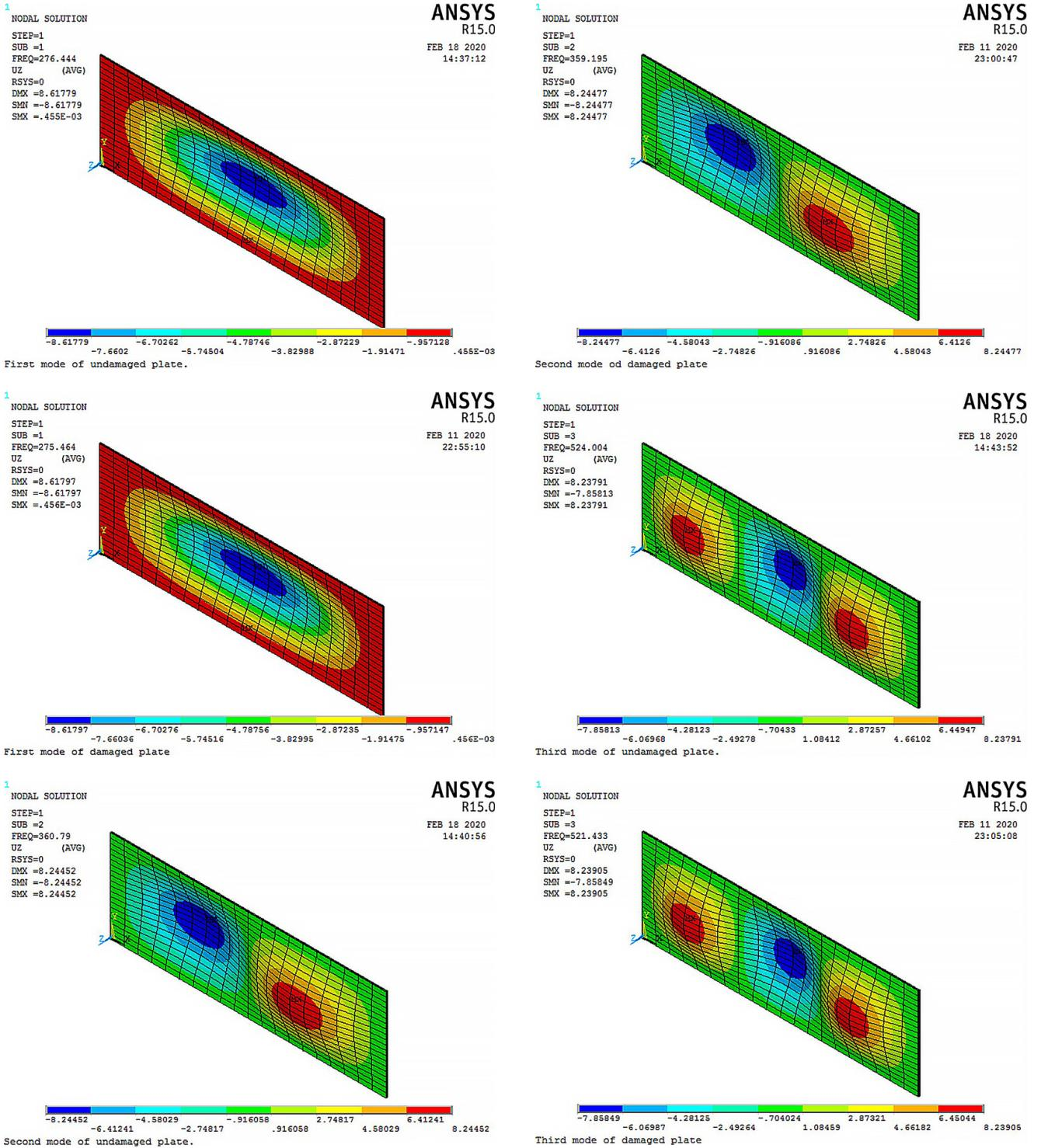
Fig. 10 The first three mode shapes of the undamaged and damaged clamped composite sandwich plate for  $\theta = 0^\circ$
