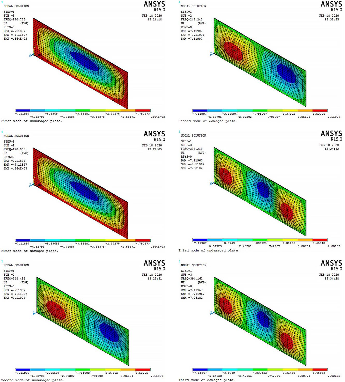
Fig. 9 The first three mode shapes of the undamaged and damaged simply supported composite sandwich plate for  $\theta = 0^\circ$
