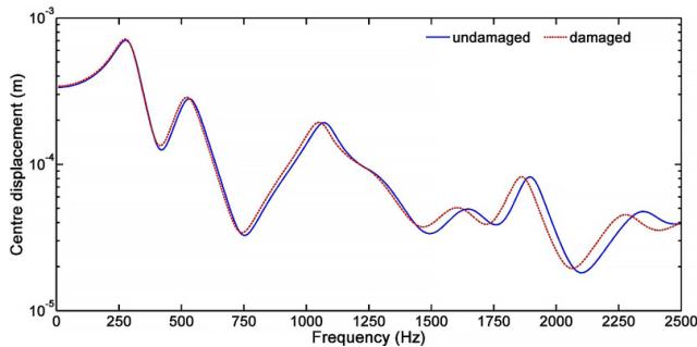
**Fig. 12** Frequency response of clamped viscoelastic composite sandwich plate in point  $P(L/2, l/2)$  for the undamaged and damaged cases with  $\theta = 0^\circ$
