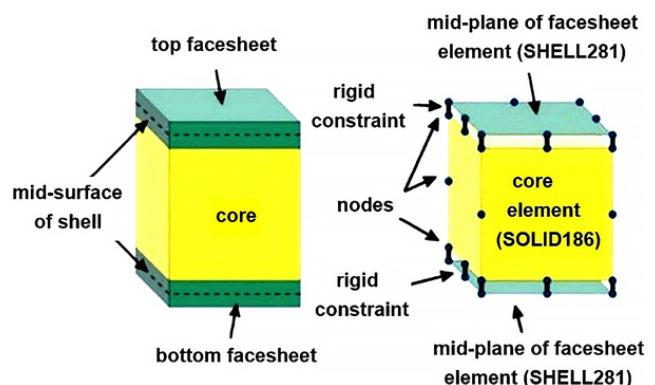
**Fig. 2** A sandwich plate and corresponding finite element model utilizing rigid constraints between the shell and solid elements: adapted from [7, 17]
