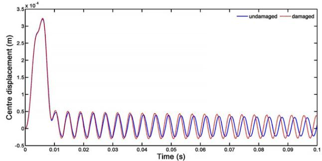
**Fig. 14** Transient response of simply supported viscoelastic composite sandwich plate in point  $P(L/2, l/2)$  for the undamaged and damaged cases with  $\theta = 0^\circ$
