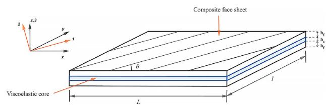
**Fig. 1** General schematic of viscoelastic composite sandwich plate
