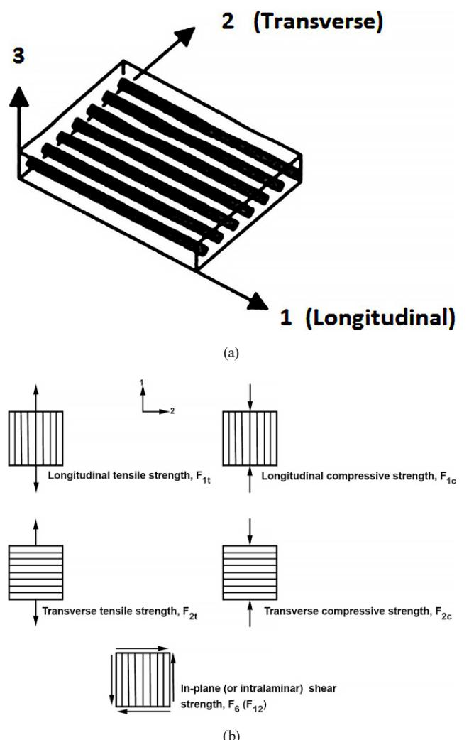
**Fig. 5** (a) Lamina and principal coordinate axes for unidirectional reinforcement, (b) Basic strength parameters of unidirectional lamina for in-plane loading: adapted from [21]
