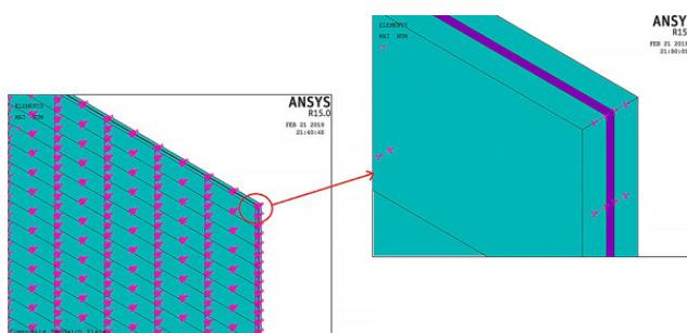
**Fig. 4** The constraints relating the motion of the face sheets to the motion of the core in ANSYS: adapted from [18]
