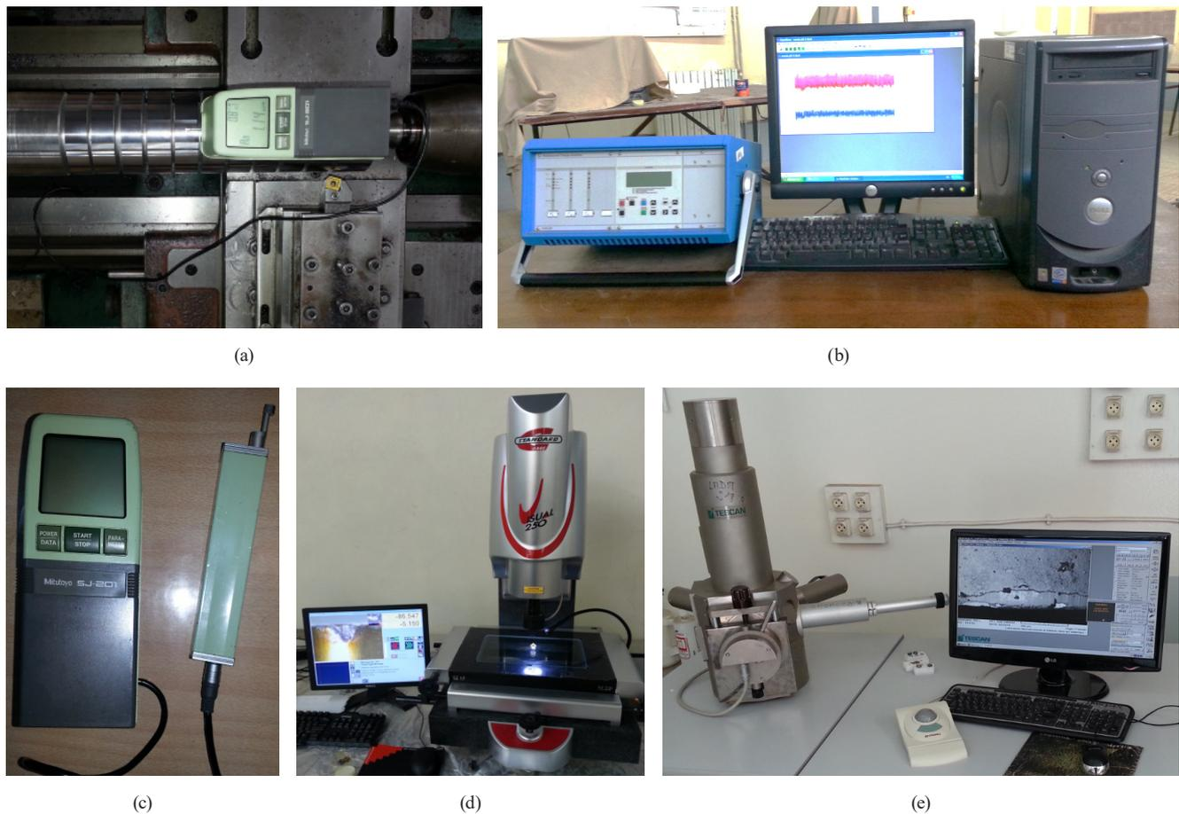
**Fig. 4** (a) Standard quartz dynamometer (Kistler 9257B), (b) Charge amplifier (Kistler 5019B130) and data acquisition system, (c) Mitutoyo Surftest-201, (d) Visual Gage 250, (e) SEM Tescan Vega TS-5130MM
