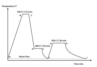
Fig. 5 Quenching follow by Tempering process
