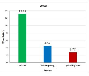
Fig. 8 Wear ratio of the specimens in different conditions
