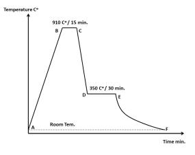
Fig. 4 Austempering process
