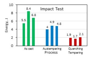
Fig. 9 Impact test results of the specimens in different conditions
