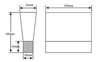
Fig. 1 Y-block specimen as cast
