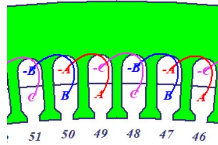
Fig. 4 Double layer fractional winding distribution
