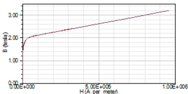
Fig. 3 B-H curve of steel\_1010
