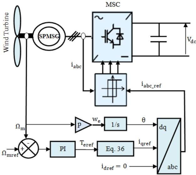
Fig. 10 Machine side converter control
