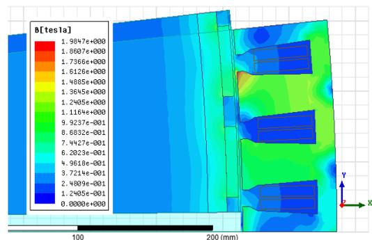
Fig. 7 Flux density distribution of the designed SPMSG
