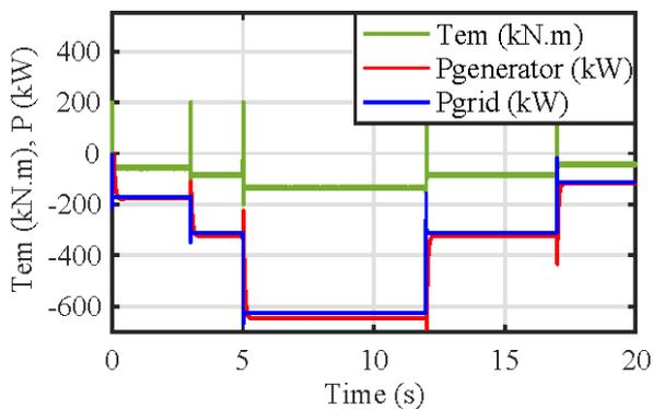
Fig. 15 Active power and electromagnetic torque
