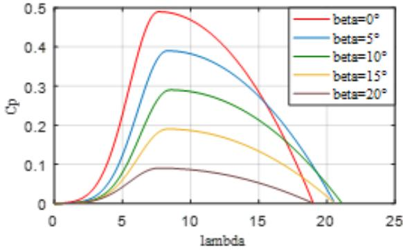
Fig. 9 Power coefficient for different values of  $\beta$
