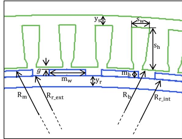
Fig. 1 Geometrical parameters of the SPMSG studied design
