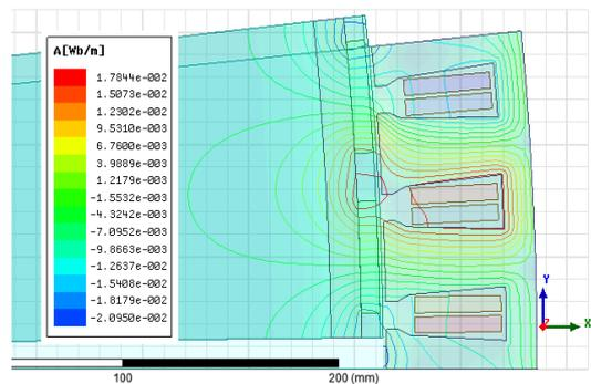
Fig. 6 Flux lines path of the designed SPMSG
