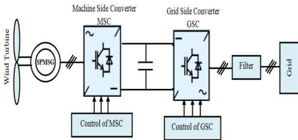
Fig. 8 SPMSG connected to the grid
