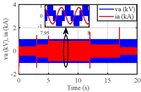
Fig. 14 Current and voltage phase of the SPMSG
