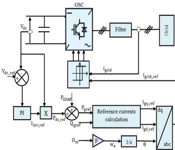
Fig. 11 Grid side converter control
