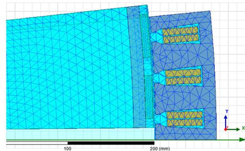
Fig. 5 Mesh analysis of the designed SPMSG
