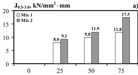
a) Post cracking flexural toughness ( $J_{0.5-3.0}$  area under the bending stress vs. mid-span deflection curves)
