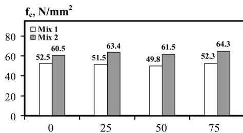
Fig. 2. Initial compressive strength at the age of 28 days (before performing the durability tests)
