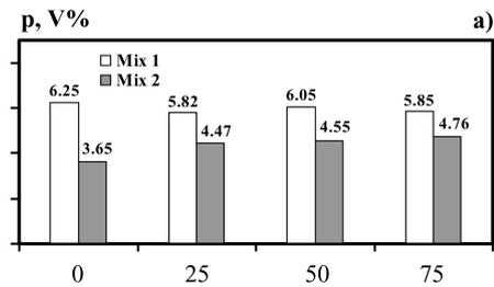
a) Apparent porosity from atmospheric water absorption test
