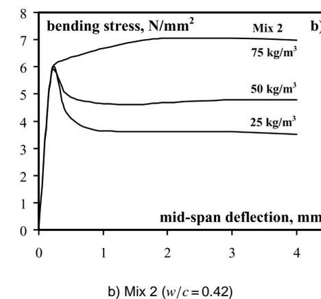
Fig. 5. Bending stress vs. mid-span deflection responses of beams tested in four-point bending
