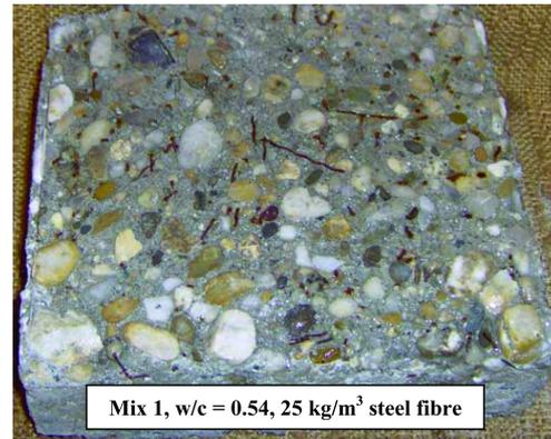
Fig. 7. Salt scaling damage of slab specimen tested according to CEN/TS 12390-9:2006 [39]
