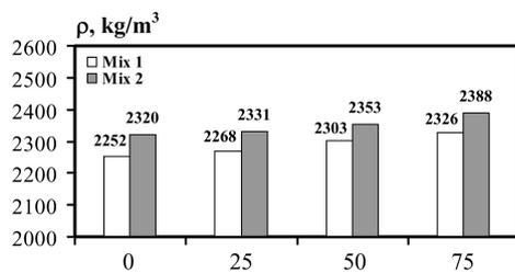
Fig. 1. Initial body density at the age of 28 days (before performing the durability tests)
