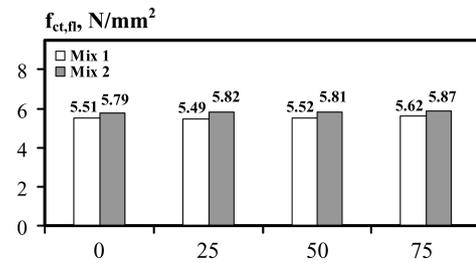
Fig. 4. Initial flexural tensile strength at the age of 28 days (before performing the durability tests)
