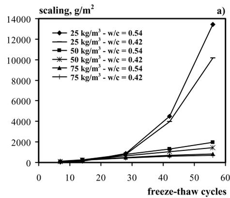
a) Linear scale of vertical axis (scaling loss)
