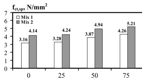
Fig. 3. Initial splitting tensile strength at the age of 28 days (before performing the durability tests)
