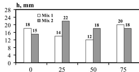
Fig. 13. Water penetration depths of 4 years old NF condition specimens recorded in watertightness tests according to EN 12390-8:2009 [42]
