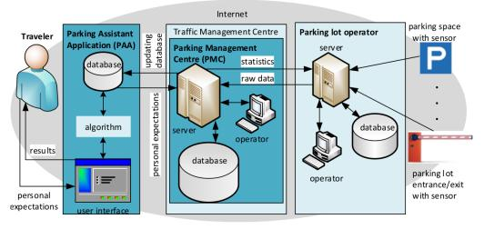
Fig. 4. Structural model of PAS (source: own)
