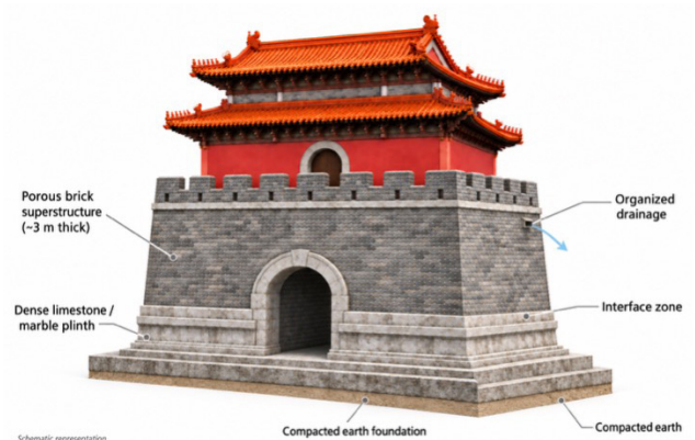
Fig. 4 Schematic diagram of the overall structure of Square City & Ming Tower and Xumizuo (Source: drawn by the author)
