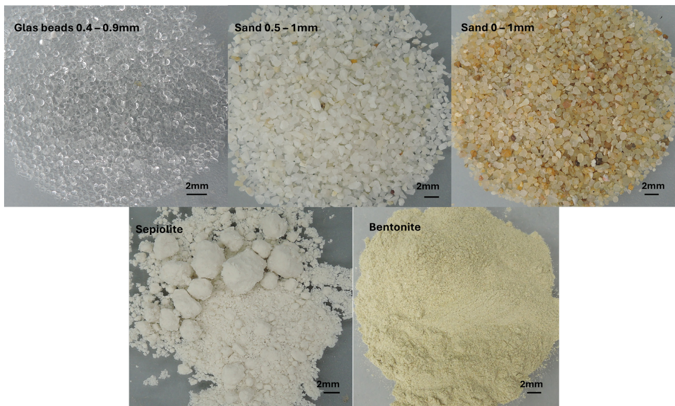
Fig. 1 Different materials used for poultice formulations. On the top, the inert fillers are displayed, on the bottom are the two clay minerals. As fillers, two different sands with grainsize between 0.5–1 mm and 0–1 mm are used, as well as homogeneous glass beads with a grainsize between 0.4–0.9 mm. Sepiolite and bentonite are used as clay minerals.
