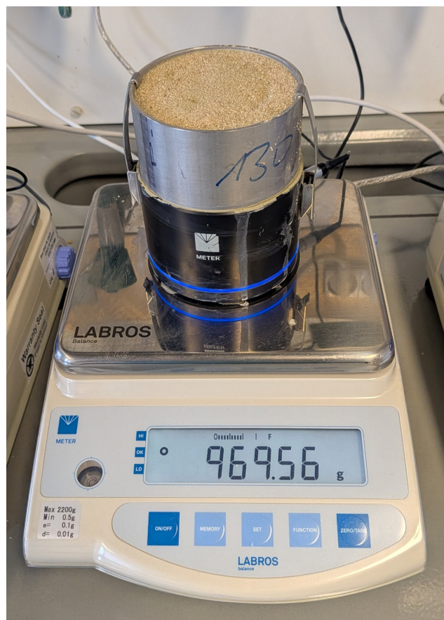
Fig. 4 Complete HYPROP setup assembled on a balance at the end of a measurement
