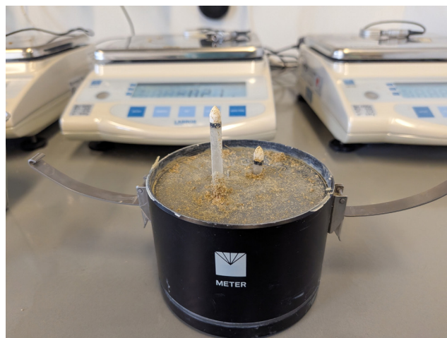
Fig. 5 HYPROP device after measurement. Here the two suction candles can be seen. The white ceramic tips are placed at different heights inside of the probe volume.
