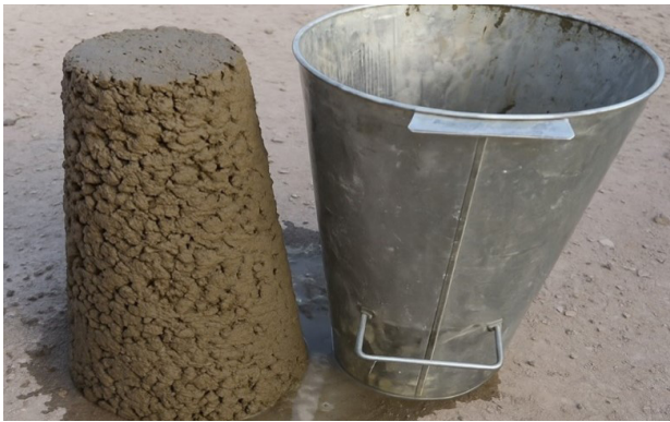
Fig. 3 slump test for fresh concrete
