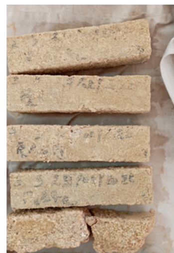
Fig. 5 Degradation and damage of specimens DM after 150 days of exposure
