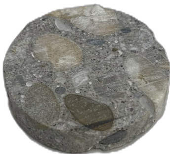
Fig. 3 Concrete specimen prepared for WRC measurement
