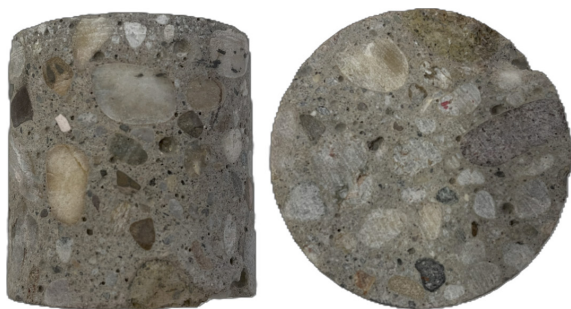
Fig. 2 Concrete specimen prepared for X-ray CT analysis
