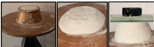
Fig. 2 Schematic representation of flow table test and buildability test
