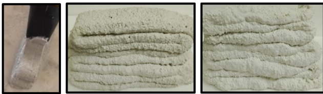
Fig. 1 Extrusion of printable concrete containing EPS
