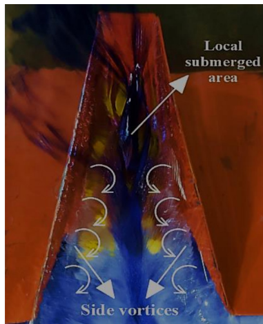
Fig. 7 Local submerged area and side eddies present in the outlet keys of the weir
