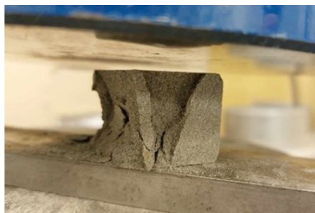
Fig. 6 Uniaxial compressive strength test
