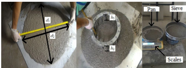
Fig. 1 Photos of the slump-flow test, J-ring test and sieve segregation test
