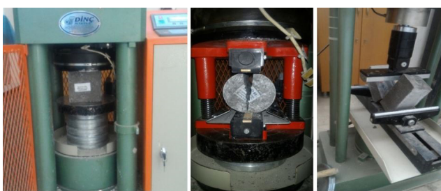
Fig. 2 Equipment used in compression test, splitting tensile test and flexural test
