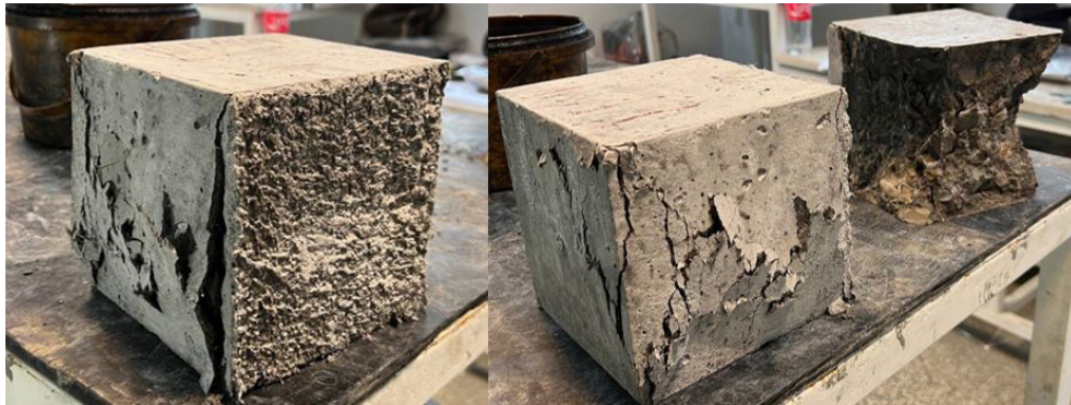
Fig. 4 Compressive strength test of cubic specimens
