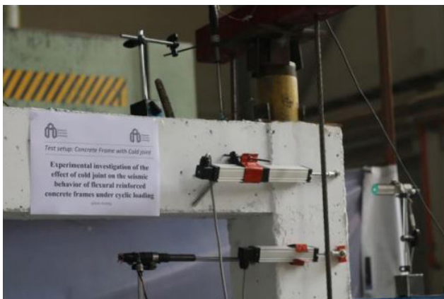
Fig. 9 Location of the LVDT in the main frame
