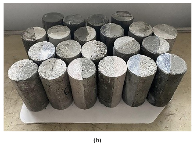
Fig. 2 Process and finished product of rock-concrete composite sample (a) The composite sample processing process (b) Rock-concrete composite specimen
