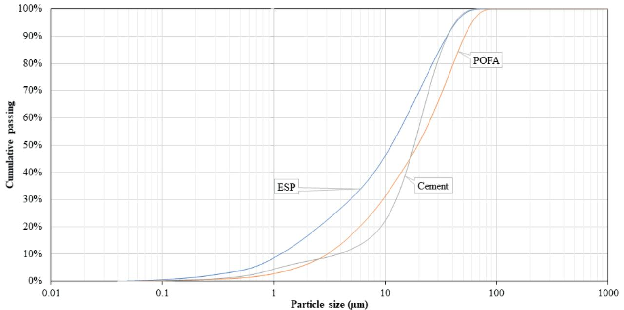
Fig. 2 Particle size distribution of binders [24]
