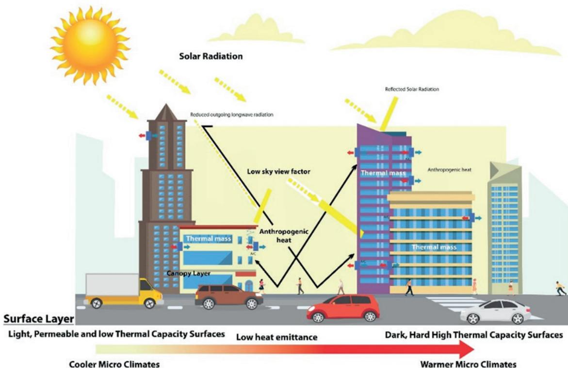
Fig. 1 Illustration of the UHI effect in an urban area [13]
