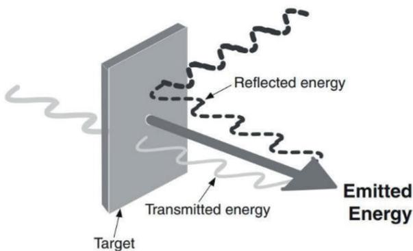
Fig. 4 Mechanism of Fluke 66 IR thermometer [32]
