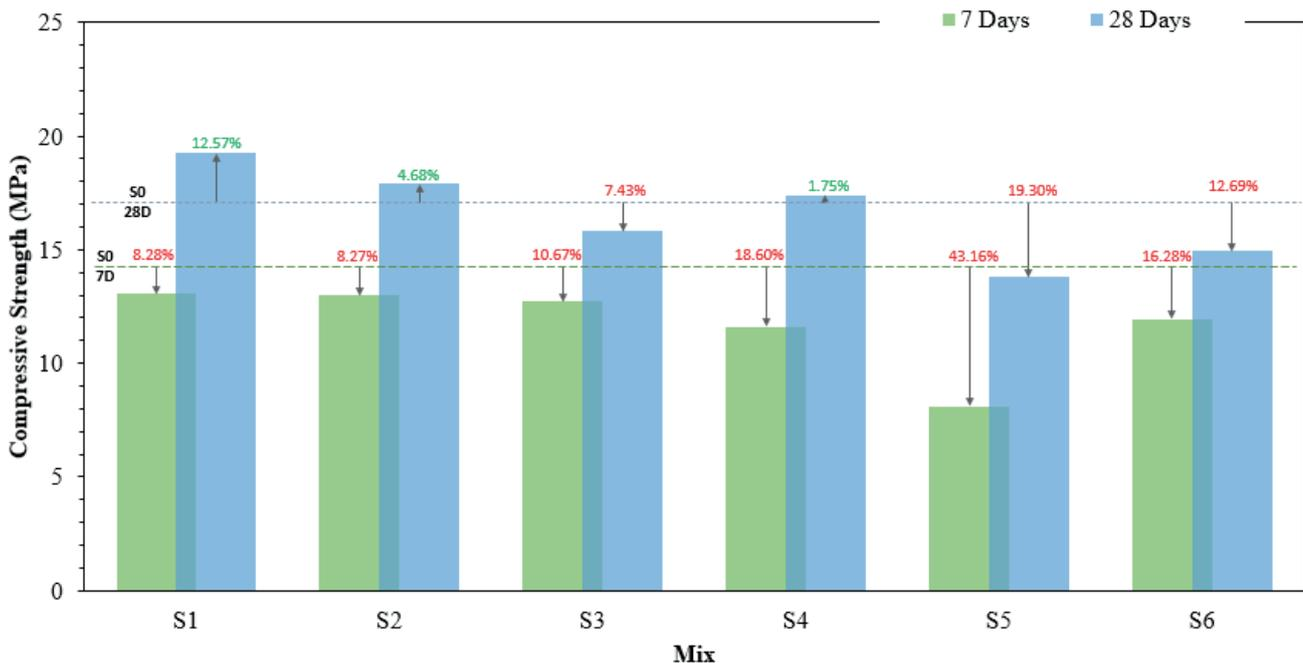
Fig. 6 Compressive strength of lightweight sustainable foamed concrete w.r.t control (S0) sample [24]
