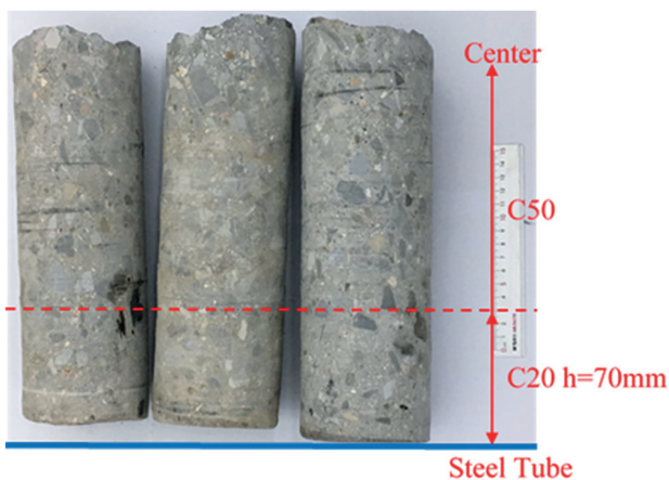
Fig. 3 Concrete segregating specimen in tube
