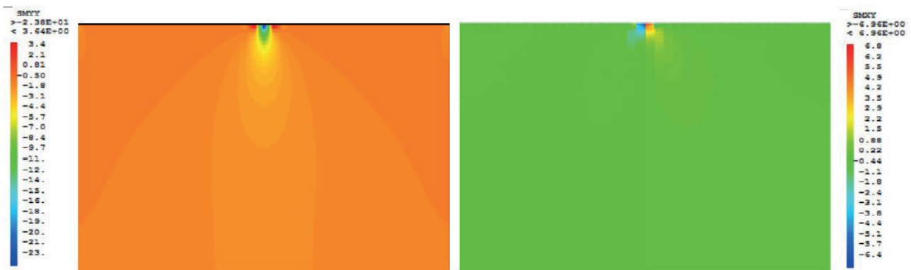
Fig. 24 Local normal (left) and shear (right) stress snapshots throughout a wall (with viscous bricks) under BC-2
