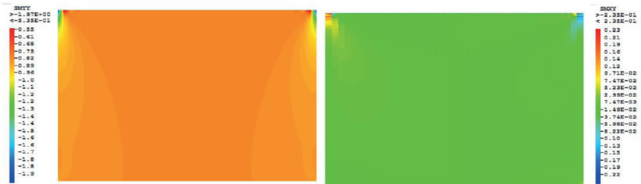
Fig. 25 Local normal (left) and shear (right) stress snapshots throughout a wall (with viscous bricks) under BC-1
