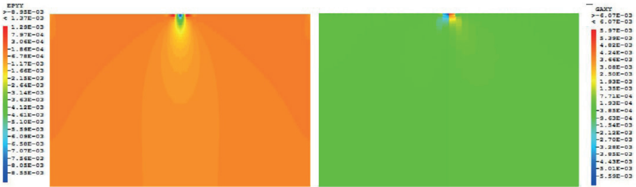
Fig. 32 Local normal (left) and shear (right) strain snapshots throughout a wall (with viscous bricks) under BC-2
