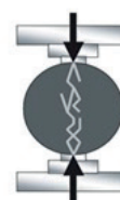
Fig. 4 The procedure of loading and performing the experiment in the indirect tensile test
