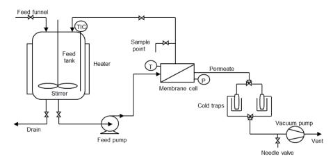
Fig. 3 Schematic representation of the setup for the pervaporation equipment.
