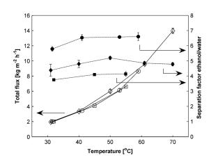
Fig. 4 Total flux (open symbols) and ethanol/water separation factor (filled symbols) as a function of temperature for ethanol/water pervaporation experiments at different feed compositions: (o) 5 wt.% ethanol, (□) 7.5 wt.% ethanol, and (◊) 10 wt.% ethanol. The lines are guidance for the eye.
