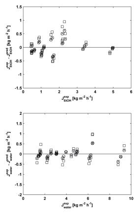
**Fig. 9** Residuals for Models 1–3 as a function of the experimental flux  $J_i^{xxp}$  for a) Ethanol and b) Water. Model 1 (o), Model 2 (x) and Model 3 ( $\Box$ ).
