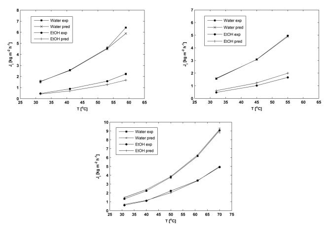
**Fig. 6** Experimental and predicted (Model 1) fluxes for ethanol and water for a) 5 wt.% EtOH, b) 7.5 wt.% EtOH and c) 10 wt.% EtOH solution as feed. The lines are guidance for the eye.
