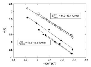
Fig. 5 Arrhenius plots for ethanol (filled symbols) and water (open symbols) for different feed compositions: (o) 5 wt.% ethanol, (□) 7.5 wt.% ethanol, nol, and (◊) 10 wt.% ethanol.
