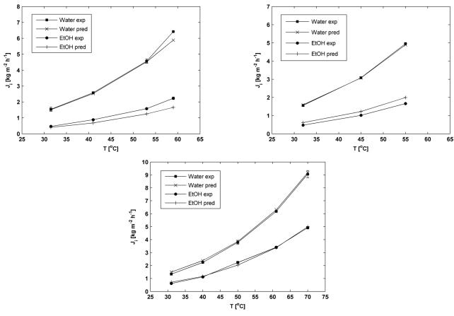
Fig. 7 Experimental and predicted (Model 2) fluxes for ethanol and water for a) 5 wt.% EtOH, b) 7.5 wt.% EtOH and c) 10 wt.% EtOH solution as feed. The lines are guidance for the eye.
