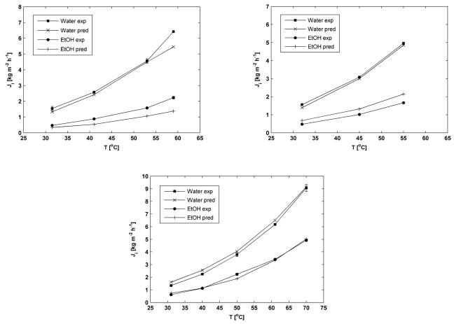
**Fig. 8** Experimental and predicted (Model 3) fluxes for ethanol and water for a) 5 wt.% EtOH, b) 7.5 wt.% EtOH and c) 10 wt.% EtOH solution as feed. The lines are guidance for the eye.
