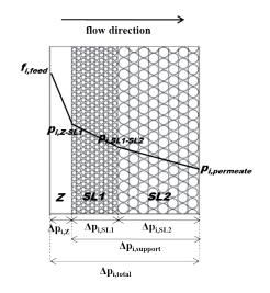
**Fig. 2** Schematic representation of the composite zeolite membrane and the fugacity profile over the zeolite film (*Z*) and support layers 1 (*SL1*) and 2 (*SL2*).
