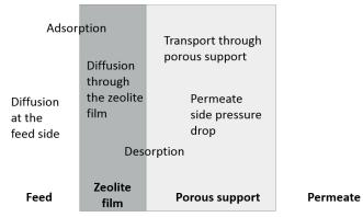
Fig. 1 Transport steps in pervaporation through zeolite membranes.
