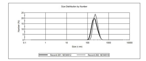
Fig. 3. Comparison of particle size distribution of nanoemulsion NE3M812 and NE3M818 with 3% of oil phase.
