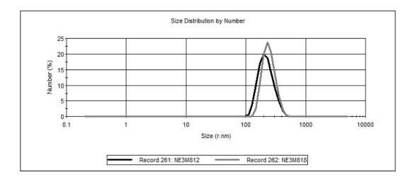
Fig. 5. Comparison of particle size distribution of nanoemulsion NE8M812 and NE8M818 with 8% of oil phase.
