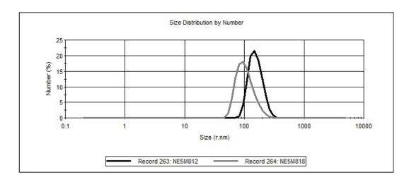
Fig. 4. Comparison of particle size distribution of nanoemulsion NE5M812 and NE5M818 with 5% of oil phase.
