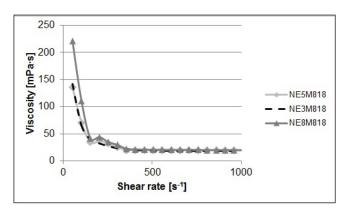
Fig. 7. Comparison of the viscosity of nanoemulsions based on Miglyol 818, at 250°C.
