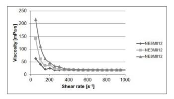
Fig. 6. Comparison of the viscosity of nanoemulsions based on Miglyol 812, at 250°C.
