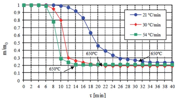
Fig. 3. Mass loss curve for the sample of agricultural biomass mixture as a function of reaction time and heating rate
