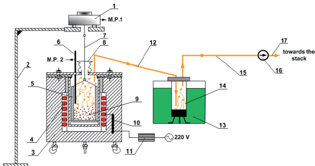
Fig. 2. The scheme of experimental facility (and metering points) for agricultural biomass pyrolysis
