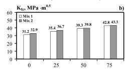
b) Fracture toughness (K<sub>Ic</sub> critical stress intensity factor)
