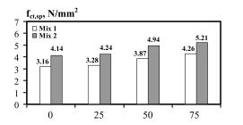
**Fig. 3.** Initial splitting tensile strength at the age of 28 days (before performing the durability tests)
