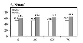
**Fig. 2.** Initial compressive strength at the age of 28 days (before performing the durability tests)
