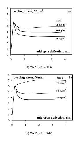
**Fig. 5.** Bending stress vs. mid-span deflection responses of beams tested in four-point bending
