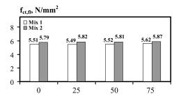
**Fig. 4.** Initial flexural tensile strength at the age of 28 days (before performing the durability tests)
