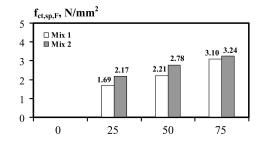
**Fig. 12.** Splitting tensile strength of specimens after 32 freeze-thaw cycles by *protocol A* (condition F)
