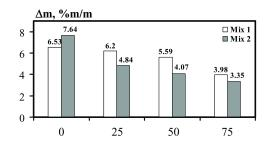
Fig. 10. Loss of mass after 32 freeze-thaw cycles by protocol A
