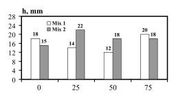
Fig. 13. Water penetration depths of 4 years old NF condition specimens recorded in watertightness tests according to EN 12390-8:2009 [42]
