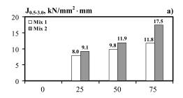
a) Post cracking flexural toughness ( $J_{0.5-3.0}$  area under the bending stress vs. mid-span deflection curves)
