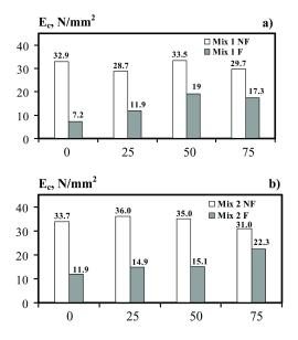
**Fig. 11.** Moduli of elasticity before (condition NF) and after (condition F) 32 freeze-thaw cycles by *protocol A*
