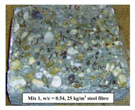
Fig. 7. Salt scaling damage of slab specimen tested according to CEN/TS 12390-9:2006 [39]
