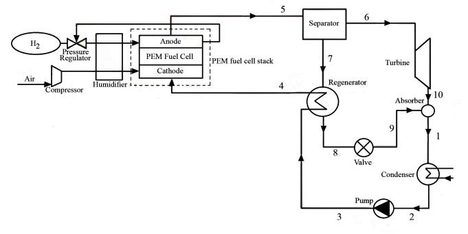
Fig. 2 Schematic of combined power system.
