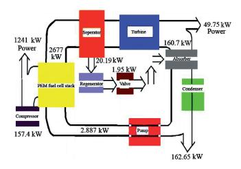
Fig. 8 The energy diagram of the combined power generation system model.
