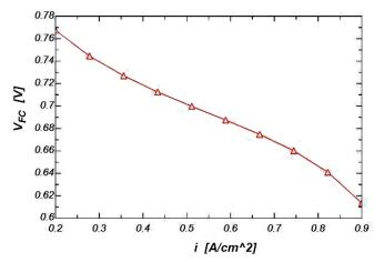
Fig. 4 The variations of the actual output voltages of the PEMFC at different current densities.
