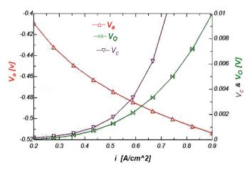
Fig. 3 Activation, concentration and ohmic, losses.
