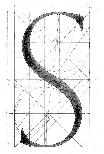
A letter S of enhanced thickness, constructed according to principles in Fig. 2, is seen in Fig. 3; the simplified construction of the joining arcs (in the middle) avoids the letter to be thinner in the middle than its upper and lower parts.
